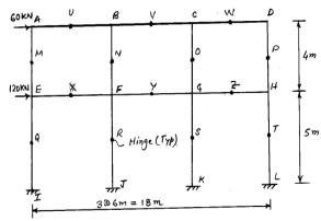
4. a) Explain the approximate method for analysis of portal frames, in case of stiff girders and state the assumptions.
