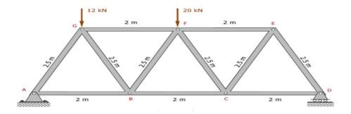
b) A truss of 12m span is loaded as shown in figure. Determine the forces in members DG, DF and EF using method of section. [7M]
