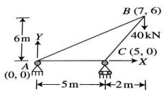
b) Find the force acting in all members of the truss shown in Figure by using method of joints.
