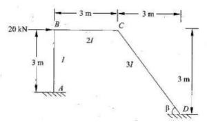
b) Analyse the frame shown in figure by slope deflection equations assume EI to be constant. Draw SFD and BMD.
